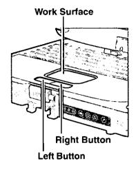
Use the touch pad to move the cursor on the display and perform normal computer operations. For instructions on how to operate, Reference "Touch Pad (Advanced)".
