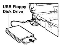
Label on the top surface, and insert the shutter-side headfirst.
